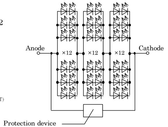
It has a protection device built in as a protection circuit against static electricity.
