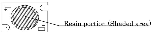
3. This product should be secured firmly by fastening an M3 screw on both sides of the product. Please be careful not to apply any stress to the product during the clamping operation. As the connection status could vary depending on materials of outer heat sink, please check thoroughly.
